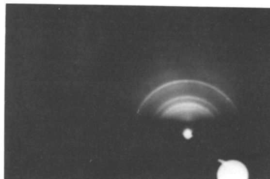
Figure 2 RHEED pattern for AlN powder heated at 1000°C.
